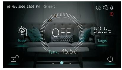
(2)In starting up interface (on/off key is in blue status), press on/off key can shut down the machine.
