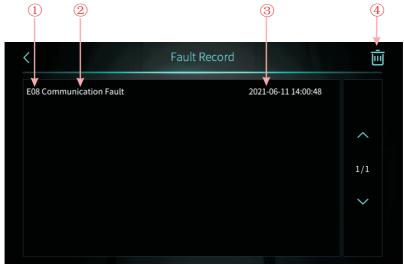
Note : ①:Fault code ②:Fault name ③:Occurrence time of the fault: Day and month hour:minute:second Note:If the current temperature is °F, occurrence time of the fault: Month and day hour: minute: second ④:Click this key to clear all fault records
